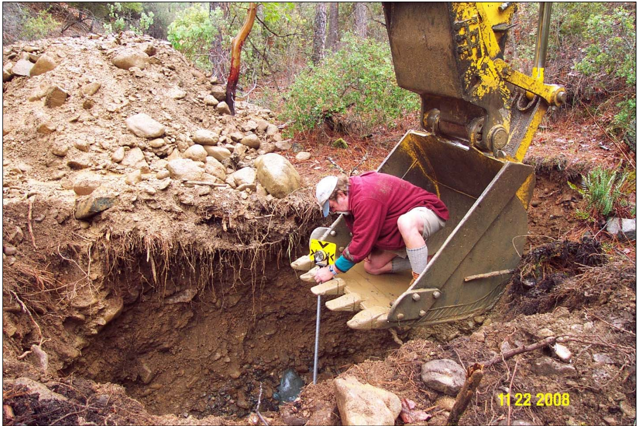
Photo 7. Surveying depth to bedrock and the water table surface in Excavation Pit # 6.
